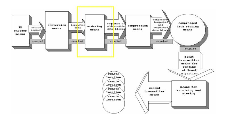
Video encoding methods organize frames into sequences of frames (data blocks) prior to compression. These frames are compressed and assigned relative time markers so that they are addressable by presentation time. The portion of the encoder that organizes the frames into sequences by assigning relative time markers (e.g., presentation time) is an example of an ordering means for placing the formatted data into a sequence of addressable data blocks.
