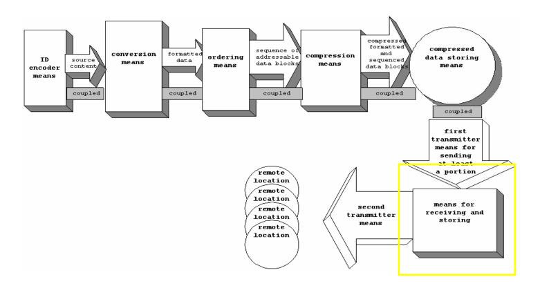
The transmitted compressed video is received via a network connection and stored as files on an array of storage devices. The network connection is an example of a means for receiving and the array of storage devices is an example of a means for storing.
