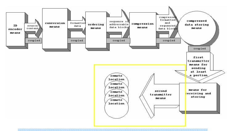
The Internet website operator transmits (e.g., streams, downloads) the video from a video server connected to the array of storage devices over the Internet to the personal computers of its users. The video server and its infrastructure is an example of a second transmitter means. The Internet connected users are an example of a plurality of remote locations.
