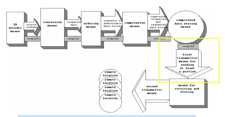
The compressed media is transmitted from the content encoding location via a file transfer method (e.g., FTP) over a network connection to the Internet website operator's distribution location. This distribution location may be managed by the website operator or by a content delivery network (CDN) or hosting provider acting on the behalf of the website operator. The network connection used to transfer the compressed media is an example of first transmitter means.
