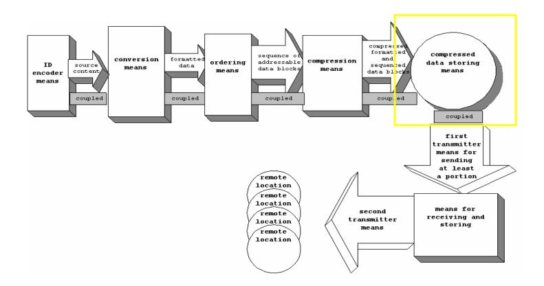
Once compressed, media is stored as files on a server. Each file stored on the server is stored with its unique identification code. The server is an example of a compressed data storing means.
