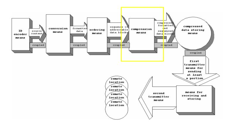
Video encoders compress video by operating on individual video frames and sequences of video frames. An Internet website operator, or an agent acting on their behalf, uses encoders by Apple, Microsoft, and/or Real to encode the media. Encoders are examples of compression means.
