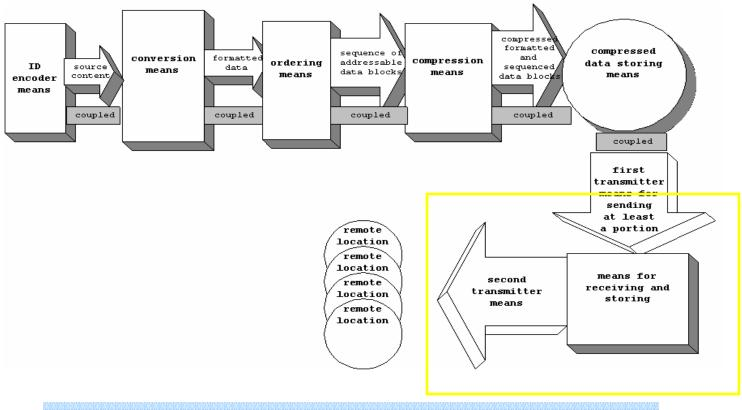
As an example, the compressed media is transmitted from servers and storage separate from the encoding servers.
