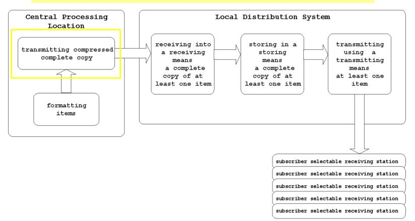
Once the media has been encoded, it is transmitted via a network connection to the website operator's distribution location. This distribution location may be managed by the website operator or by a content delivery network (CDN) or hosting provider acting on the behalf of the website operator. This is an example of transmitting compressed audio/video information from the central processing location.
