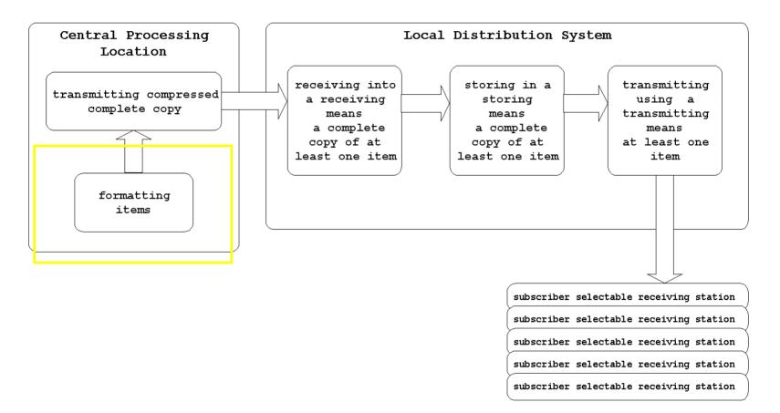
Physical media (e.g., videotape) is encoded (digitized and compressed). An Internet website, or an agent acting on their behalf, encodes the physical media prior to distribution to customers. Encoding is an example of formatting items as compressed digitized data.
