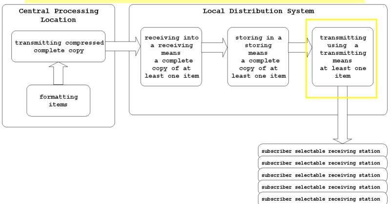
From the distribution location, the Internet website operator transmits the encoded media from a video server connected to the array of storage devices over the Internet to the personal computers of their customers. The video server and its infrastructure is an example of a transmitting means.
