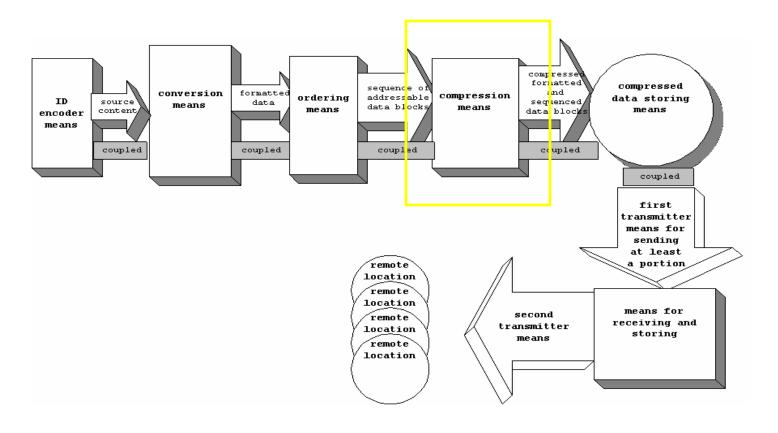
Video encoders compress video by operating on individual video frames and sequences of video frames. An online education provider, or an agent acting on their behalf, uses encoders by Apple, Microsoft, and/or Real to encode the media. Encoders are examples of compression means.
