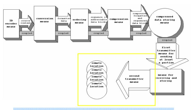
The online education provider transmits the media from a video server connected to the array of storage devices over the Internet to the personal computers of its students. The video server and its infrastructure is an example of a second transmitter means. The Internet connected students are an example of a plurality of remote locations.
