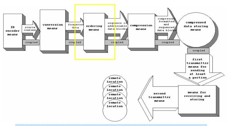
Video encoding methods organize frames into sequences of frames (data blocks) prior to compression. These frames are compressed and assigned relative time markers so that they are addressable by presentation time. The portion of the encoder that organizes the frames into sequences by assigning relative time markers (e.g., presentation time) is an example of an ordering means for placing the formatted data into a sequence of addressable data blocks.
