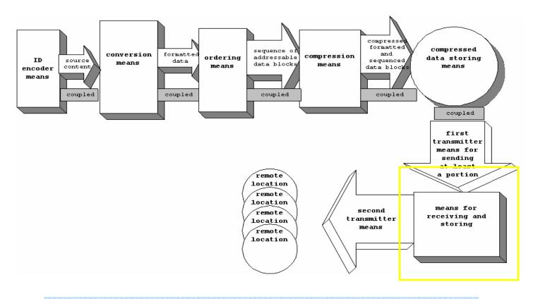
The transmitted compressed media is received via a network connection and stored as files on an array of storage devices. The network connection is an example of a means for receiving and the array of storage devices is an example of a means for storing.
