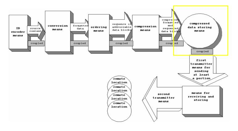
Once compressed, media is stored as files on a server. Each file stored on the server is stored with its unique identification code. The server is an example of a compressed data storing means.
