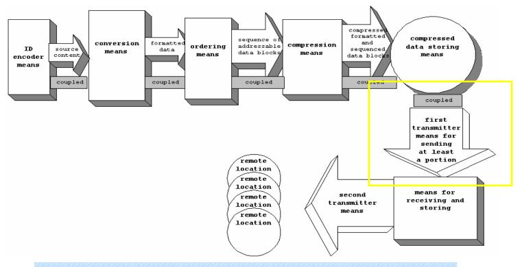
The compressed media is transmitted from the content encoding location via a file transfer method (e.g., FTP) over a network connection to the online education provider's distribution location. This distribution location may be managed by the online education provider or by a content delivery network (CDN) or hosting provider acting on the behalf of the online education provider. The network connection used to transfer the compressed media is an example of first transmitter means.
