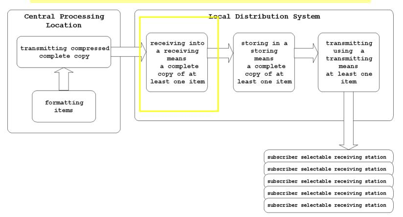
The encoded media is received via a network interface card (NIC) at the distribution location. The network interface card is an example of a receiving means.
