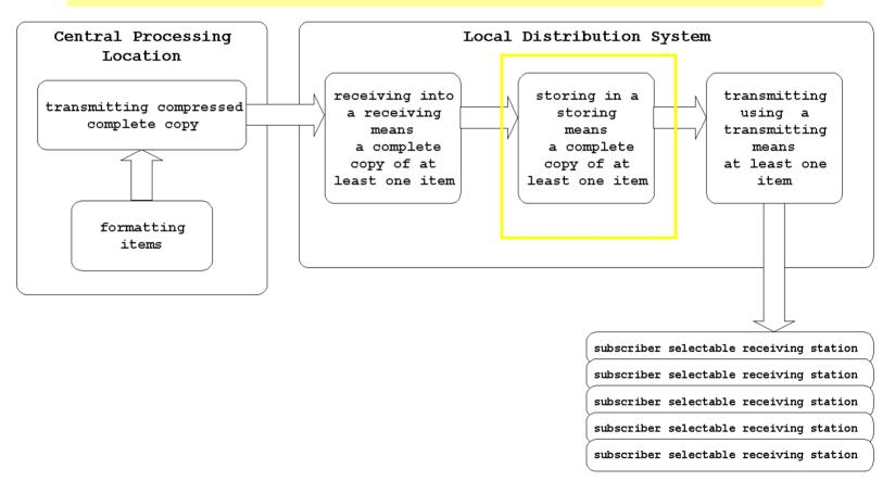
The received encoded media is stored on an array of storage devices. The array of storage devices is an example of a storing means at a local distribution system.
