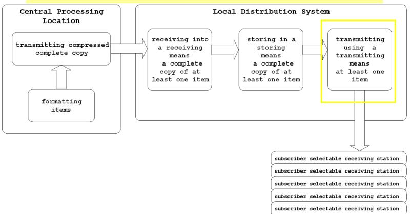
From the distribution location, the online education provider transmits the encoded media from a video server connected to the array of storage devices over the Internet to the personal computers of their students. The video server and its infrastructure is an example of a transmitting means.
