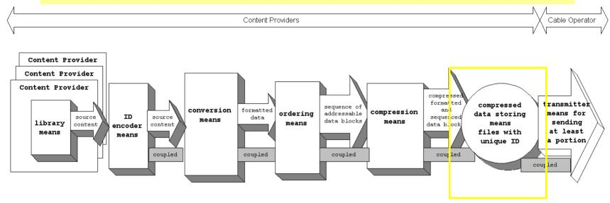
Once compressed, media is stored as files on a server. Each file stored on the server with its unique identification code. A server is an example of a compressed data storing means.
