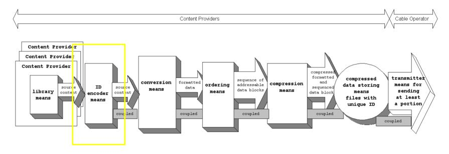
A tape operator(s) retrieves physical media (e.g. a videotape) from a tape library to be encoded. A unique file name will be used to identify the encoded media on a server after it has been encoded. The tape operator(s) and the encoding software are one example of an identification encoding means for retrieving information and for assigning a unique identification code to the retrieved information.
