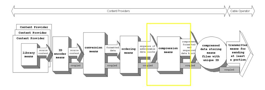
Video encoders, such as MPEG-2 encoders, compress video by operating on individual video frames and sequences of video frames. MPEG-2 encoders are examples of compression means.
