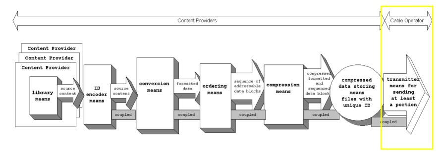
Media is transmitted as files from the content provider to the cable operator via satellite or terrestrially. Once at the cable headend, the cable operator uses the cable plant to transmit the media (either in an MPEG-2 format or in an analog format) to the subscribers' set-top box via the cable network. The cable network is an example of a transmitter means.
