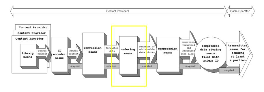
Video encoding methods organize frames into sequences of frames (data blocks) prior to compression. These frames are compressed and assigned relative time markers so that they are addressable by presentation time. The portion of the encoder that organizes the frames into sequences by assigning relative time markers (e.g., presentation time) is an example of an ordering means for placing the formatted data into a sequence of addressable data blocks.
