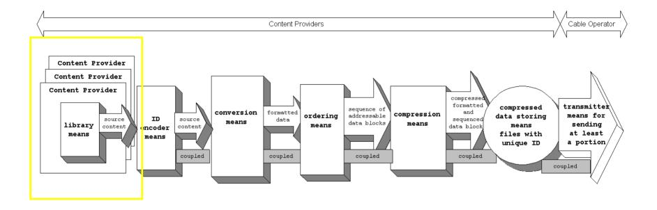
Cable operators receive and deliver media from a variety of different content providers. Each content provider, acting on behalf of the cable operator, receives physical media such as videotapes at their respective receiving department from a number of sources, each of these sources having a media storage library, the media storage library being a library means. The sources' media storage libraries are examples of a plurality of library means for storing items containing information.
