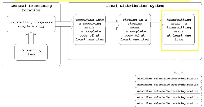
The available stored media is delivered by the cable operator to the subscriber set-top boxes via, for example, an HFC network. The HFC network is an example of a transmitting means.
