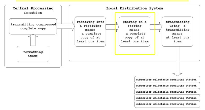
The received compressed media is stored on a server in the cable headend. The server is an example of a storing means at a local distribution system.
