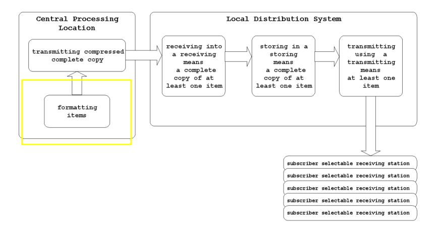
At a facility independent from the cable operator, content providers, acting on behalf of the cable operator, encode physical media and produce compressed digital copies of the physical media. Encoding is an example of formatting items as compressed digitized data.
