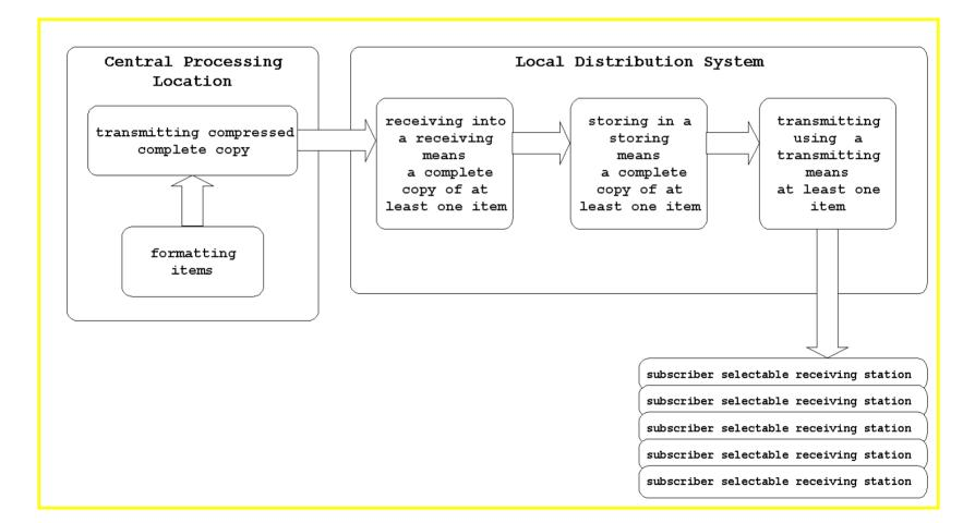
A cable video on demand system delivers media (e.g., movies) to subscriber set-top boxes. This media may be in a compressed digital format and is transmitted to the cable operators by content providers. This is an example of a method of distributing audio/video information.
