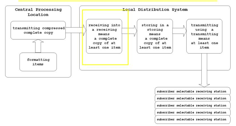
A cable operator receives the compressed media via a satellite receiver at a cable headend. The satellite receiver is an example of a receiving means at a local distribution system.
