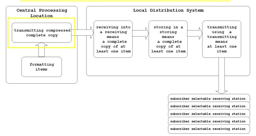
The content provider transmits the compressed media via satellite from its central processing facility to a cable operator headend. This is an example of transmitting compressed audio/video information from the central processing location.
