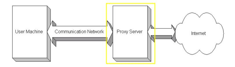
The hot spot gateway is in communication with the user machine and the Internet. The hot spot gateway is connected to the wireless based network via a network adapter in order to receive messages from the user machine. The hot spot gateway is an example of a proxy server in communication with a user machine and the global computer network.
